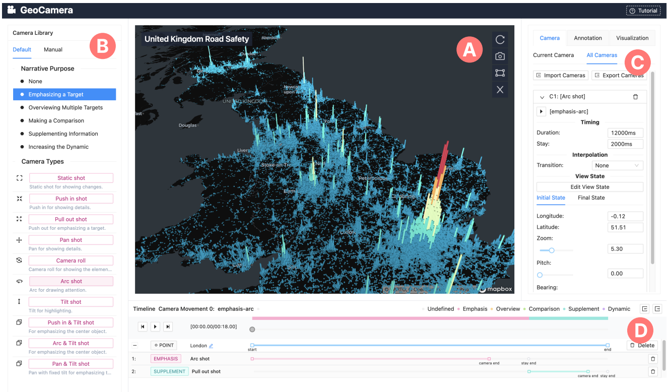
Figure 1: The user interface of GeoCamera: (A) previewer of camera movements in the geographic visualization with geospatial targets selection, (B) library of camera shots classified by narrative purposes, (C) camera and visual configurations and crafted examples, and (D) location-camera hierarchical timeline.
